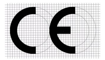
The CE marking shall have a vertical dimension of at least 5mm.
