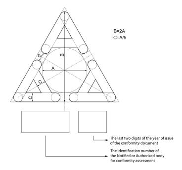
The height of the mark must be determined by the B height of the mark which may have only values of standard numbers rounded up, to the order of magnitude R10 expresses in millimetres (mm), as per Serbian standard SRPS A.A0.001 – Standard numbers, numerical values and definitions.
